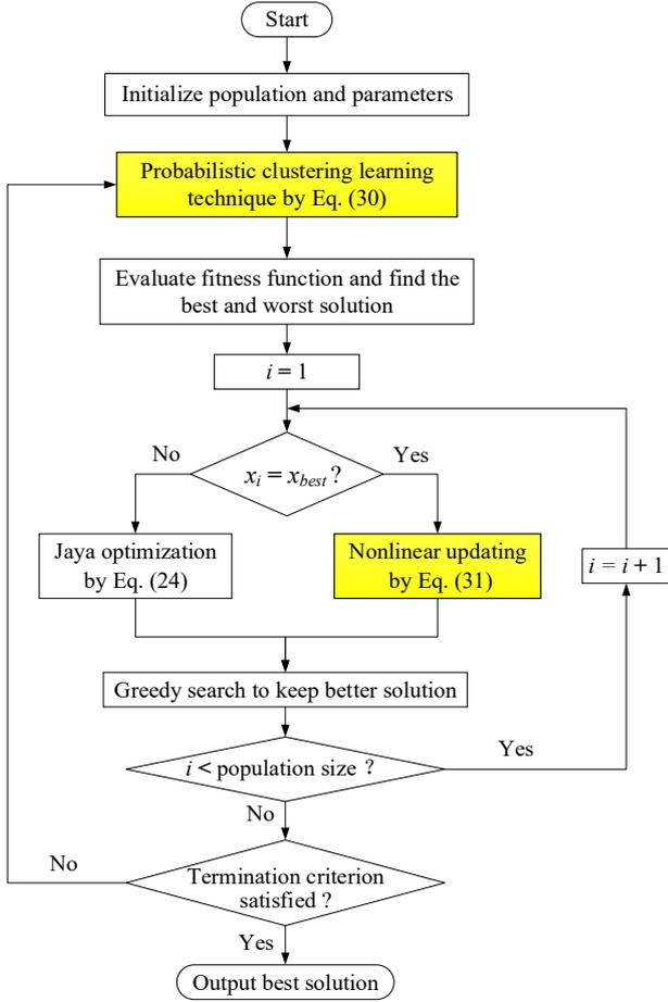
Fig. 3 The flowchart of proposed M-Jaya algorithm
