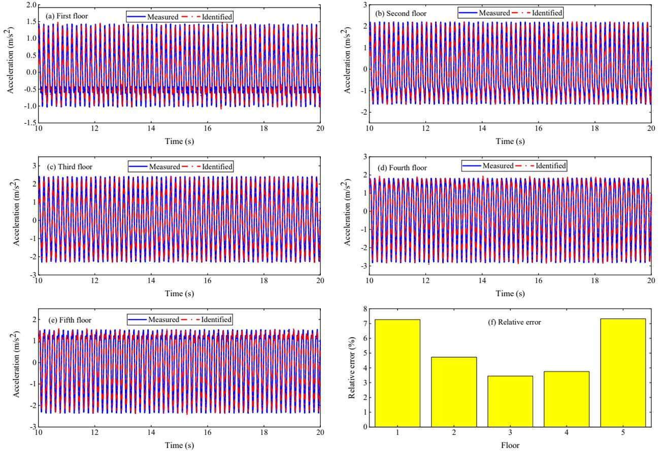
Fig. 17 The measured and predicted acceleration time histories of frame model in case 2: (a) first floor; (b) second floor; (c) third floor; (d) fourth floor; (e) fifth floor; (f) relative error
