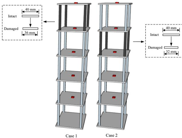
Fig. 14 Two damage cases of steel frame model
