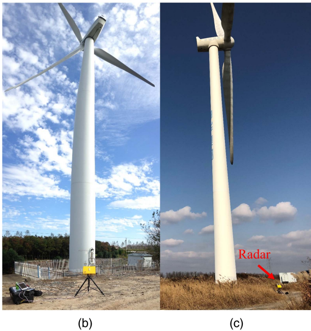
Fig. 5. Field testing with use of IR sensor: (a) IR measurement and test setups; (b) Tower A; and (c) Tower B.
