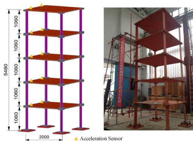
Figure 9. Schematic diagram and the test model of the 5-DOF structure system.
